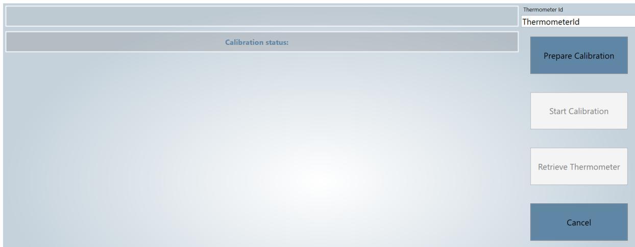
**Step 5:** Once you’ve made sure the sensor is ON and its LED light is blinking green, tap on the “**Prepare Calibration**” button.
