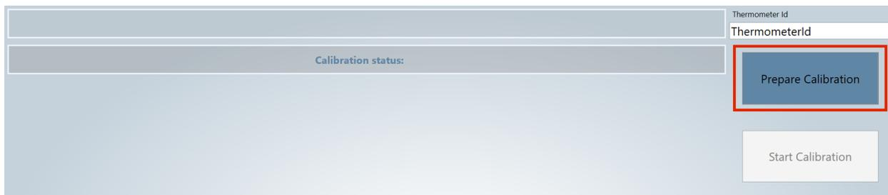
**Step 6:** Hitting the “Prepare Calibration” button will open AccuVax’s doors, revealing two empty slips. Once the doors of the AccuVax are open, place the NIST traceable calibration sensor in either one of the slips, with the blue button facing up and inwards. Please double check the LED light is blinking green.
