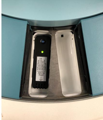
**Step 7:** After placing the sensor in one of the empty slips, tap the “**Start Calibration**” button. Once the “Start Calibration” button is tapped, the doors of the AccuVax will close and the Temperature Calibration will start.
